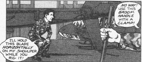
One of the simplest work aids to make and use requires only a broom handle and a hose clamp like the ones used on your bird's battery vent hoses.
