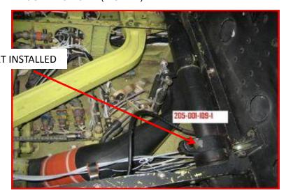
NOTE ON THE INCORRECT PART THERE IS APPROXIMATELY 90+ DEGREES BETWEEN THE "CLAMPING BOLT" (INSET C) AND THE "MOUNTING BOLT" (INSET D).
