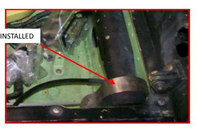
NOTE IN THE CORRECT PART THERE IS APPROXIMATELY 45 DEGREES BETWEEN THE "CLAMPING BOLT" (INSET A) AND THE "MOUNTING BOLT" (INSET B).
