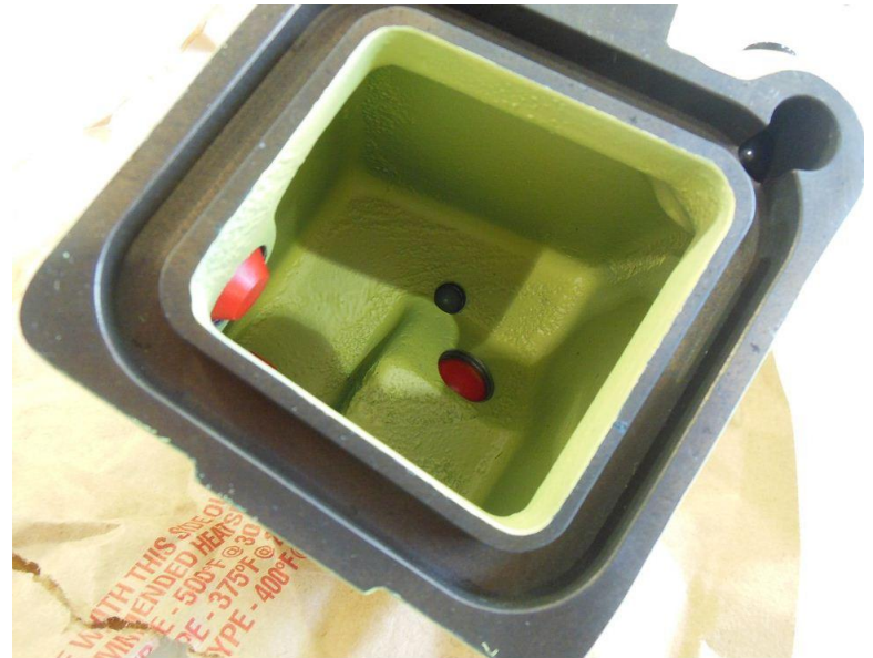
Non-conforming (yellow-green primer coating inside housing)
